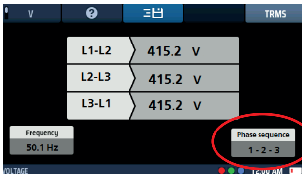
Fig 36: Voltage phase rotation
