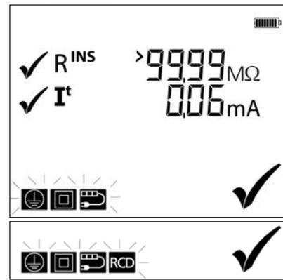
**NOTE :** High touch leakage measurement on faulty equipment can trip the supply RCD
