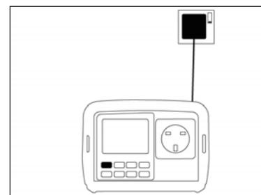
Connect the Instrument to the mains supply using the mains plug test lead (for mains powered leakage and RCD testing)
