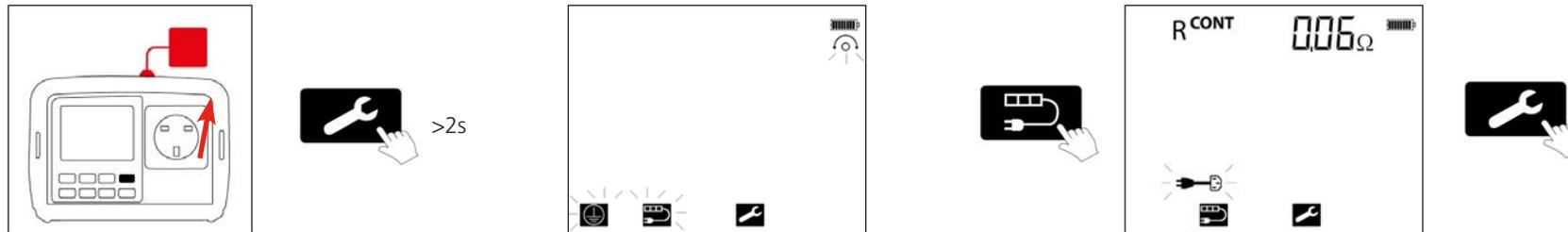
To NULL the resistance of the P1 continuity test lead
