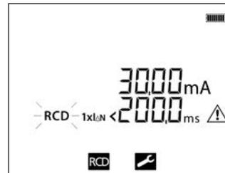
iii) Press RCD button to change from 30 mA to 10 mA
