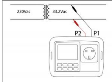
Connect both the P1 and P2 test leads to the circuit to be measured.
