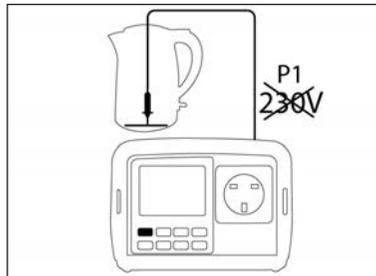
Connect the P1 test lead to socket P1 on the Pat100 and the probe to exposed metalwork. Ensure the probe is NOT connected to a 230V source.
