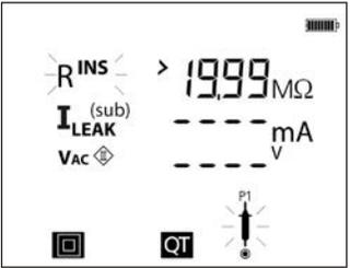
Example 3 – Class II touch leakage test using the Substitute (or alternative) method.
