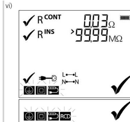
NOTE : For power cords longer than 5m the test can be re-run with a 1.0Ω pass limit by pressing the
