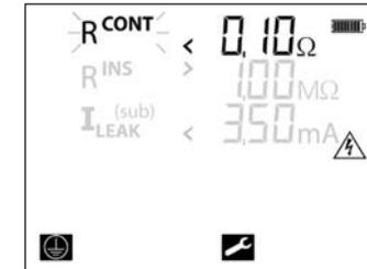
v) Keep pressing the TEST GROUP button to select the test to be changed
