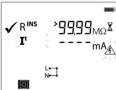
If the L to N short circuit symbol shows, user must check whether there is a true short circuit. Press Class II button to proceed but there is a risk of damage or tripping of protective devices.
