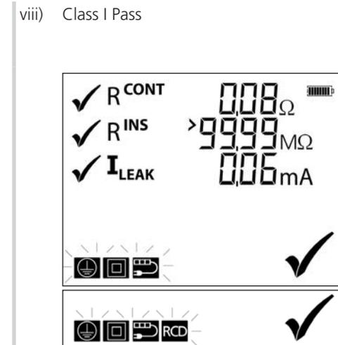
NOTE: If the contact symbol
