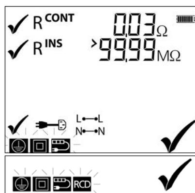
**NOTE:** Multiple earth continuity tests can be carried out by pressing the QT button during the continuity test, and pressing it again for each new continuity test. See Page 13
