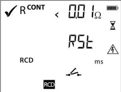
v) Press TEST button on RCD
