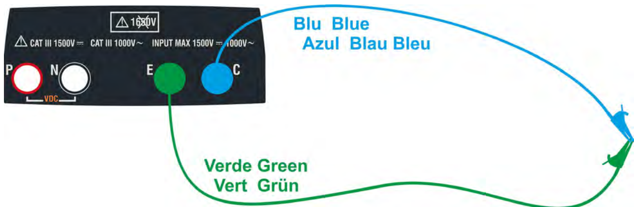
Fig. 4: Compensation of the measuring cables resistance
