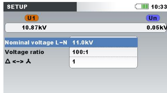
Figure 4.17: Voltage ratio for 11 kV / 110 kV transformer example
