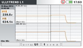
Figure 4.19: Voltage and current trend (dual mode)
