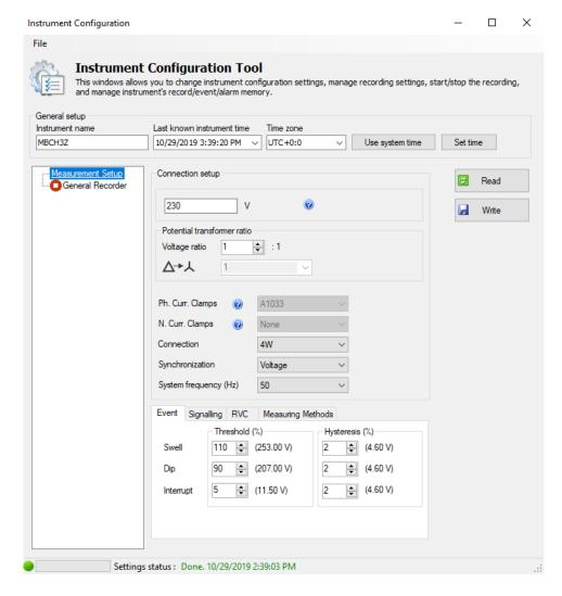
Figure 5.28: Remote Instrument Configuration form
