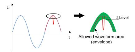
Figure 6.27: Transients trigger detection (envelope)
