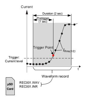
Figure 6.23: Current Level Triggering (Inrush)
