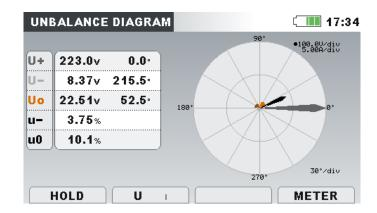
Figure 4.37: Unbalance diagram screen
