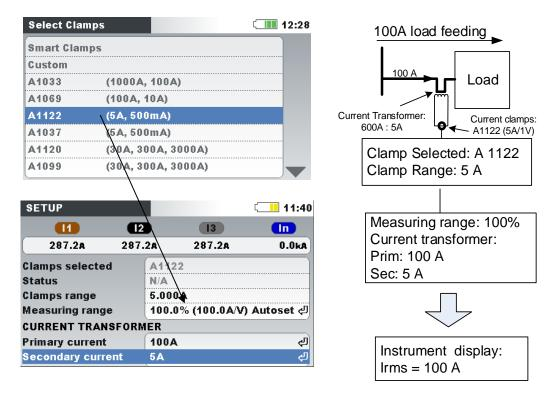
Figure 5.17: Current clamps selection for indirect current measurement
