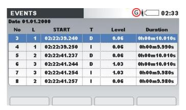
Figure 4.55: Voltage event in detail view screen
