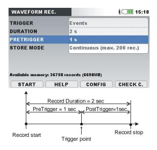
Figure 6.20: Triggering and pre-triggering description
