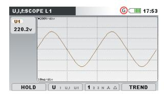
Figure 4.12: Voltage only waveform
