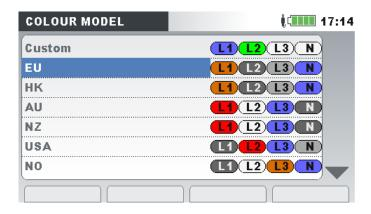
Figure 4.77: Colour representation of phase voltages
