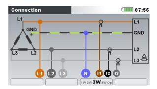
Figure 5.5: Choosing 3-phase 3-wire system on instrument
