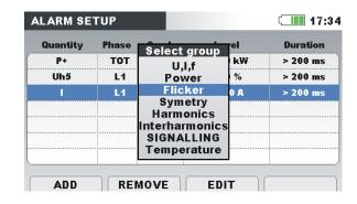
Figure 4.67: Alarm setup screens
