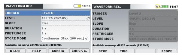
Figure 4.48: Waveform recorder setup screen
