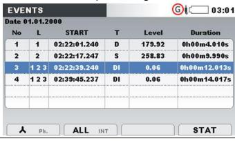
Shows poly-phase voltage interrupts only, according to the IEC 61000-4-30 requirements. START time and Duration in table is referenced to voltage interrupt only.
