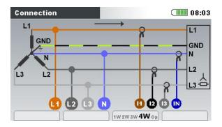
Figure 5.3: Choosing 3-phase 4-wire system on instrument
