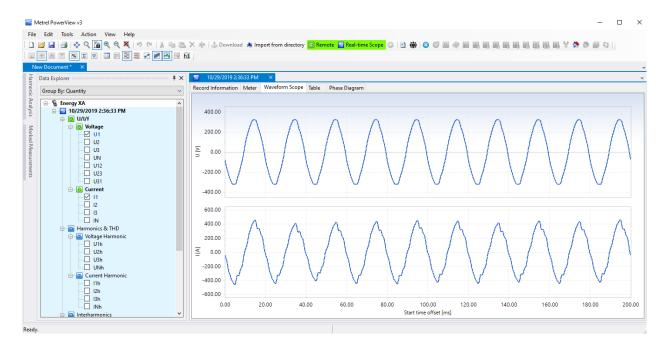
Figure 5.27: Real time scope window in remote connection, with several channels selected
