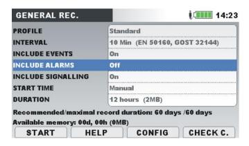
Figure 4.46: General recorder setup screen
