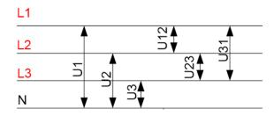
Figure 6.1: Phase and Phase-to-phase (line) voltage
