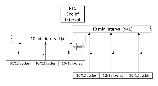
Figure 6.16: Synchronization and aggregation of 10/12 cycle intervals
