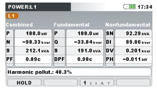
Figure 4.24: Detailed power measurements at phase L1
