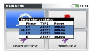
Figure 5.20: Automatically recognised clamps status
