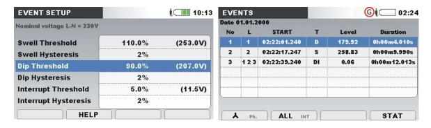
Figure 6.13:Voltage dip related screens on the instrument
