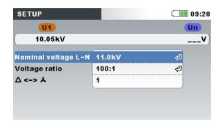
Figure 5.13: Voltage ratio for 11 kV / 110 kV transformer example
