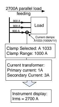
Figure 5.16: Parallel feeding of large load
