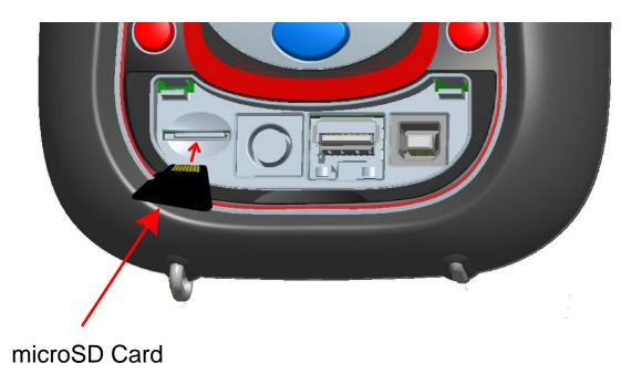
Figure 4.4: Inserting microSD card
