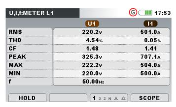
Figure 4.10: U, I, f meter phase table screens (L1, L2, L3, N)
