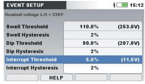
Figure 6.24: Waveform recorder setup for triggering on voltage events
