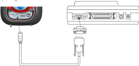
Figure 5.21: Connecting printer DPU 414 with instrument
