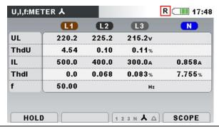
Figure 4.63: U,I,f meter screen in recalled snapshot record
