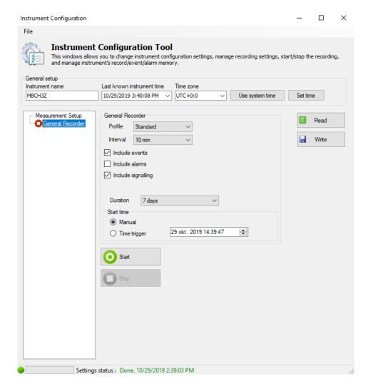
Figure 5.29: Remote Recorder configuration
