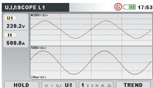
Figure 4.15: Voltage and current waveform (dual mode)
