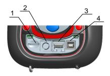
Figure 3.3: Side connector panel
