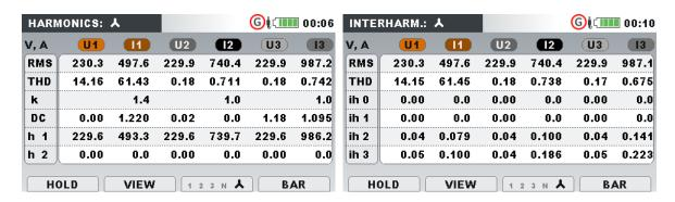
Figure 4.30: Harmonics and interharmonics (METER) screens
