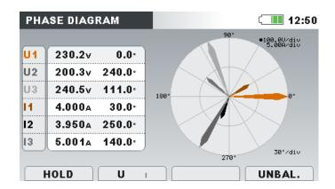
Figure 4.36: Phase diagram screen
