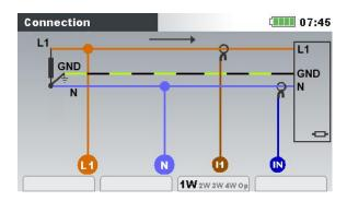
Figure 5.9: Choosing 1-phase 3-wire system on instrument
