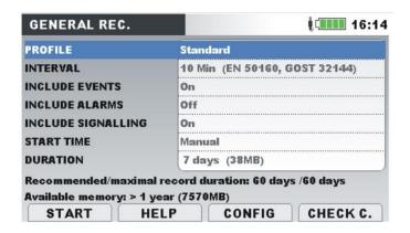
Figure 6.30: Predefined EN50160 recorder configuration
