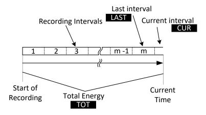
Figure 6.7: Instrument energy counters
