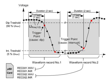
Figure 6.21: Voltage Event Triggering
