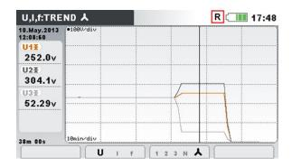
Figure 4.61: Viewing recorder U,I,f TREND data
