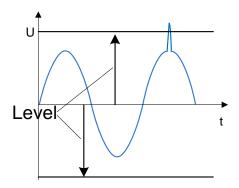
Figure 6.28: Transients trigger detection (envelope)
