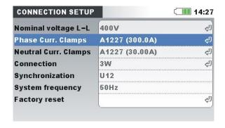
Figure 5.19: Automatically recognised clamps setup
