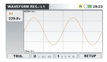
Figure 4.49: Waveform recorder capture screen
