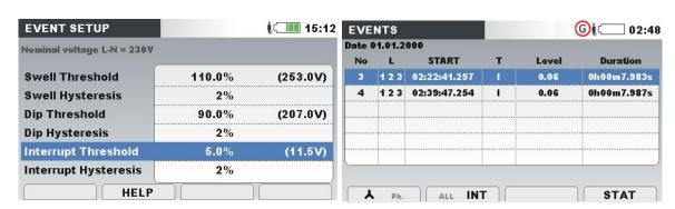
Figure 6.14:Voltage interrupts related screens on the instrument
