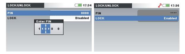
Figure 4.75: Lock/Unlock screen
