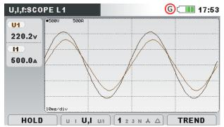
Figure 4.14: Voltage and current waveform (single mode)
