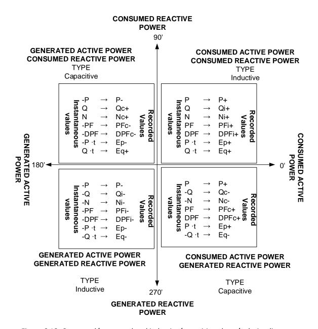
Figure 6.18: Consumed/generated and inductive/capacitive phase/polarity diagram
