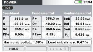
Figure 4.25: Detailed total power measurements
