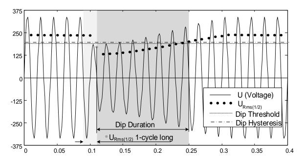
Figure 6.11: $U_{Rms(1/2)}$  1-cycle measurement
