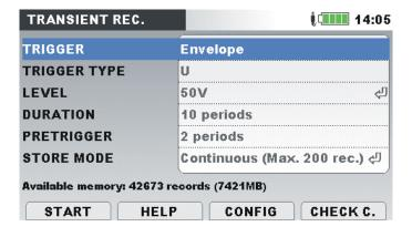
Figure 4.51: Transient recorder setup screen
