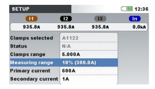
Figure 5.18: Selecting 10% of current clamps range
