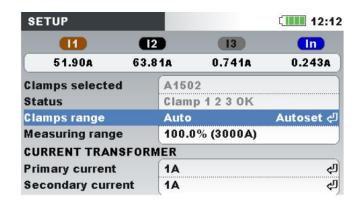
Figure 5.15: Smart current clamps auto range selection
