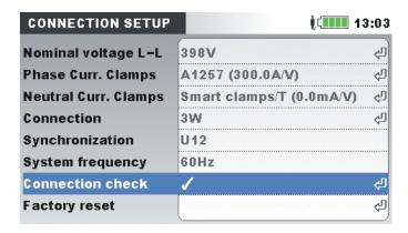
Connection check mark can be marked with OK ( $\checkmark$ ) or Fail ( $\nearrow$ ) sign and indicate overall connection status:
