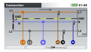
Figure 5.11: Choosing 2-phase 4-wire system on instrument
