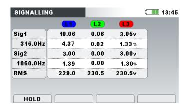
Figure 4.43: Signalling meter screen
