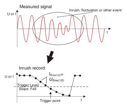
Figure 6.25: Level triggering
