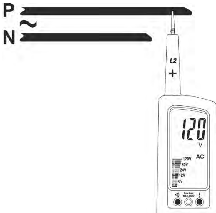
Fig. 5: 1-wire AC Voltage detection
