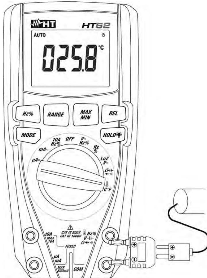
Fig. 9: Use of the instrument for Temperature measurement
