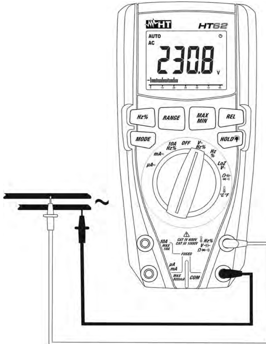
Fig. 3: Use of the instrument for AC voltage measurement
