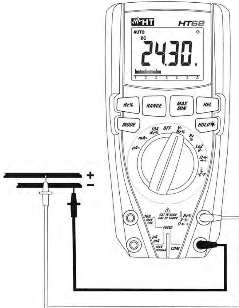
Fig. 2: Use of the instrument for DC voltage measurement
