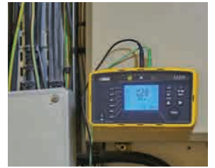
Magnetized casing for magnetic mounting.
